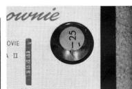
12 After the cover is on and locked, hold the exposure lever down until 25 on the dial of the footage indicator is at the index. Now you can take pictures.
