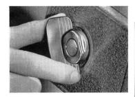
1 First of all, give the winding key a few turns before you start to load, to make sure that the motor is not run down. Never load the camera if the motor is run down.
