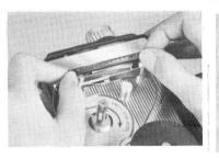
**5** Let the film follow the line with the arrow from the bottom of the film spool to the gate. Slide the film down into the gate; that is, between the pressure pad and aperture plate (pointed out in 3 above).
