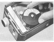
8 Place the spool on the take-up spindle so that the instructions are up. Turn the spool slightly, if necessary, so that the spool fits all the way down with the end of the spindle projecting through the hole in the spool.
