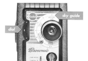
The Exposure Guide, located on the side of the camera, shows the proper lens opening to use under daylight or flood lamp conditions with Kodachrome Film Daylight Type or Kodachrome Film Type A. Slip the little silver card packed with each roll of film into the guide; one side of the card is for daylight exposures, the other side for flood lamp exposures.
