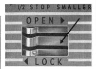
2 Next, press in on the center spring leaf of the cover latch (shown by the arrow in the picture above) and at the same time slide the latch as far as it will go in the direction indicated to open.
